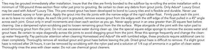
If skips or voids in the grout joint are discovered after final clean-up they can be filled by applying new grout directly over the old.
