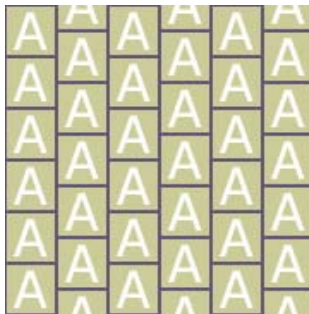
Brick/Ashlar-Vertical Half Drop Vertical
