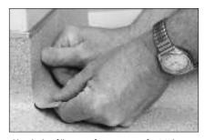
Check the fill piece for accurate fit. Make any minor adjustments to the plug as necessary to fill the space correctly. Remove the fitted fill piece and apply the appropriate adhesive. Reposition the fill piece and apply seam sealer.
